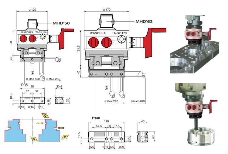
On the dovetail slide, in addition to the P95 - P140 universal toolholder for boring and facing, a wide range of toolholders of the Testarossa TRM 63/80 and TRM 80/125 heads are applicable.
